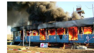
Figure 1: Full-scale fire test of rail car for Munich subway. [2]
